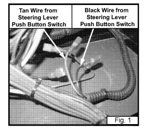
Locate the tan and black wiring from the steering lever hydraulic push button switch and disconnect both leads from the tractor's harness.
