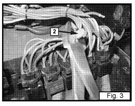
Crimp a blue female spade terminal (item 2) onto the brown wire leading into the connector.
