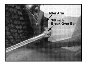
Insert a 3/8 inch drive break over bar into the square hole and rotate hydro pump idler arm counter clockwise.
