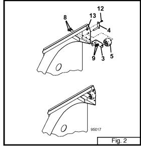
roller pin along with the roller mount (item 3, Fig. 2).
