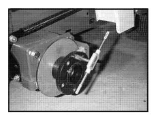
Install puller as shown with light oil on the bolt threads. Tighten the bolts evenly so they do not bind up in the puller. Do not use a jaw type or T-bar puller with a center point screw as you may damage the axle.
