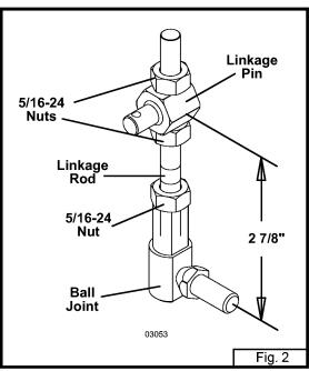
• Thread two 5/16-24 nuts (item 4), one on each end of a linkage rod (item 16). Thread a linkage pin (item 18) on the longer threaded end of rod and a ball joint (item 7) on the shorter threaded end. Adjust linkage
