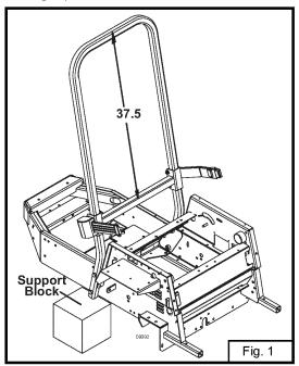
Attach seat belt (item 7) to the cross member end brackets in a position that allows belt to be routed outside of seat's side members and under arm rest. Secure with .5-13 x 1.5 bolts, spacers, nylon washers and lock nut (items 8-10 & 3). Refer to illustration for the correct position of spacers and nylon washers. If Grammer seat is installed, disregard seat belts included in this kit.
