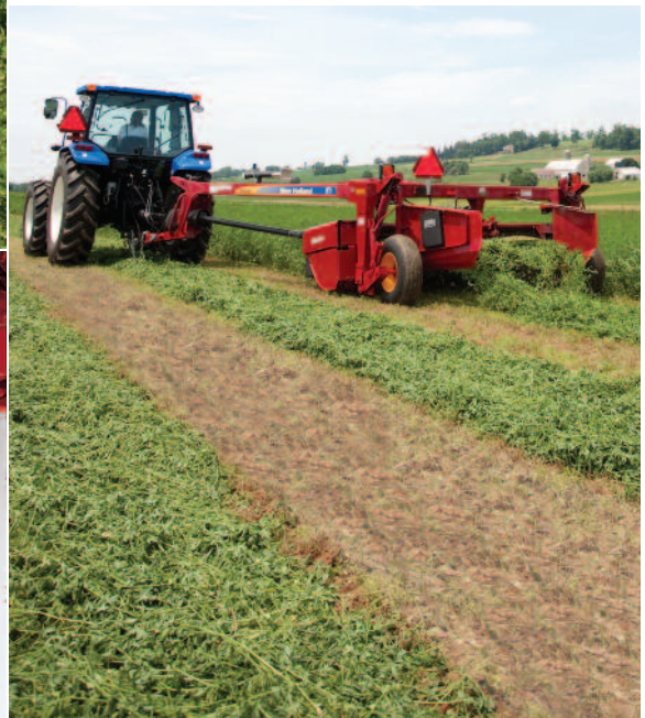
The Discbine header is suspended independently from the trail frame, allowing it to closely follow changing ground contours and reducing stubble damage and skid shoe wear.
